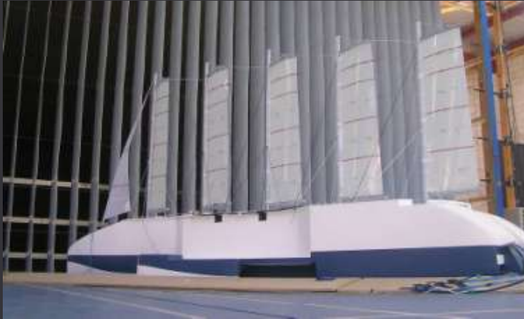
Patented rig concept during wind tunnel trials (STX Europe)
